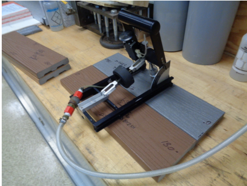
Photo No. 3 Slip Resistance Test Setup
