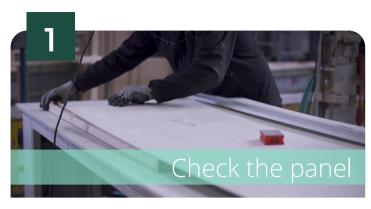
After measuring the wall and determining the dimensions, **put the slab horizontally** on a cutting table (polished side on top).
