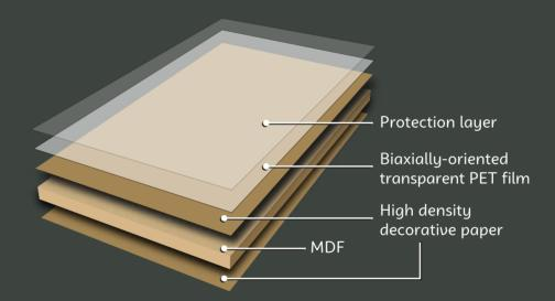
Polylac panel is made by pressing a high density decorative paper / pp to MDF. A specially developed biaxially-oriented transparent PET film is then laminated on the surface to protect it from external factors.
