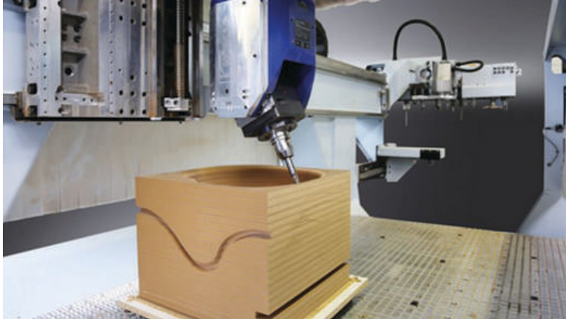
Mould preparation with HOMAG CNC
